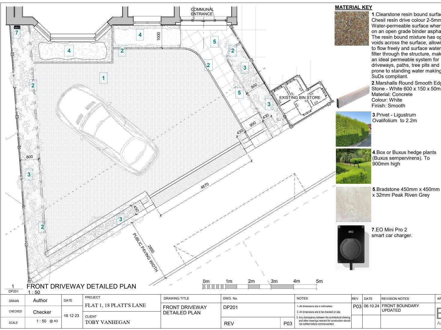
**1**.Clearstone resin bound surfacing. Chesil resin drive colour 2-5mm. Water-permeable surface when laid on an open grade binder asphalt. The resin bound mixture has open voids across the surface, allowing air to flow freely and surface water to filter through the structure, making it an ideal permeable system for driveways, paths, tree pits and areas prone to standing water making it
