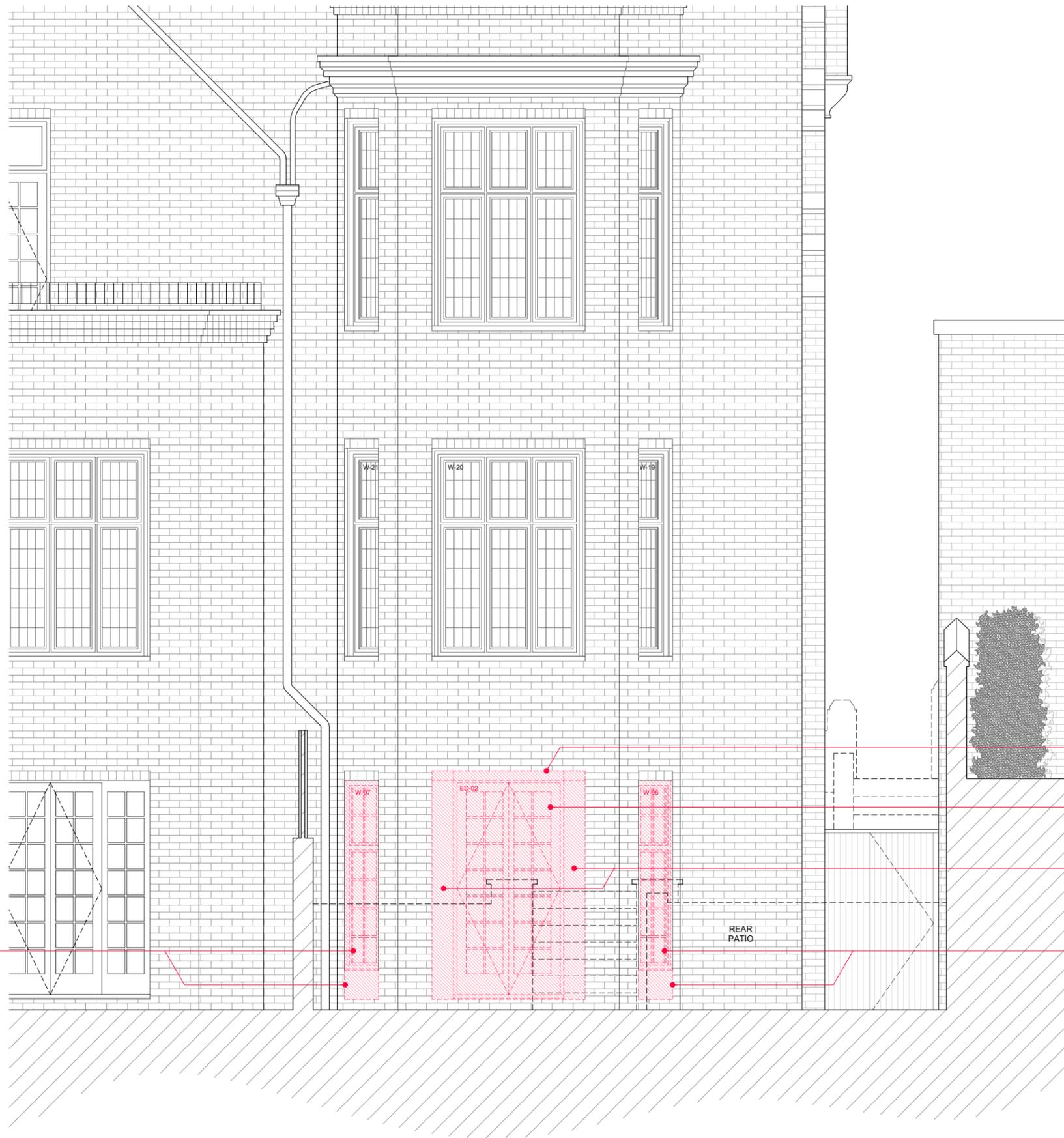
LOWER GROUND FLOOR EXISTING TIMBER FRAMED GLAZED REAR WINDOWS TO BE REMOVED, TO BE REPLACED WITH NEW WINDOW OPENINGS TO BE ENLARGED DOWN TO GROUND LEVEL, TO MATCH HEIGHT OF ADJACENT DOOR OPENING
