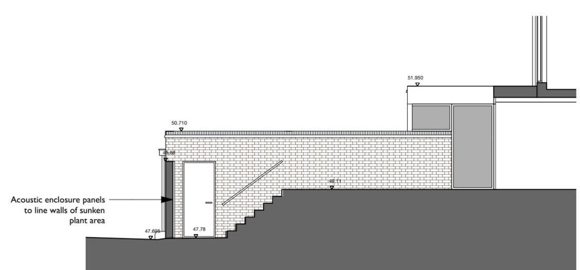
05 - Proposed Section/Elevation
