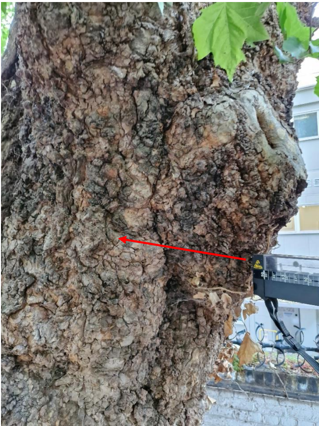
Photo 11: Showing location of resistance drill profile 2 carried out at 4m to the south, below the historical wound towards the centre of the stem. Approximate projection of drill shown by a red arrow.
