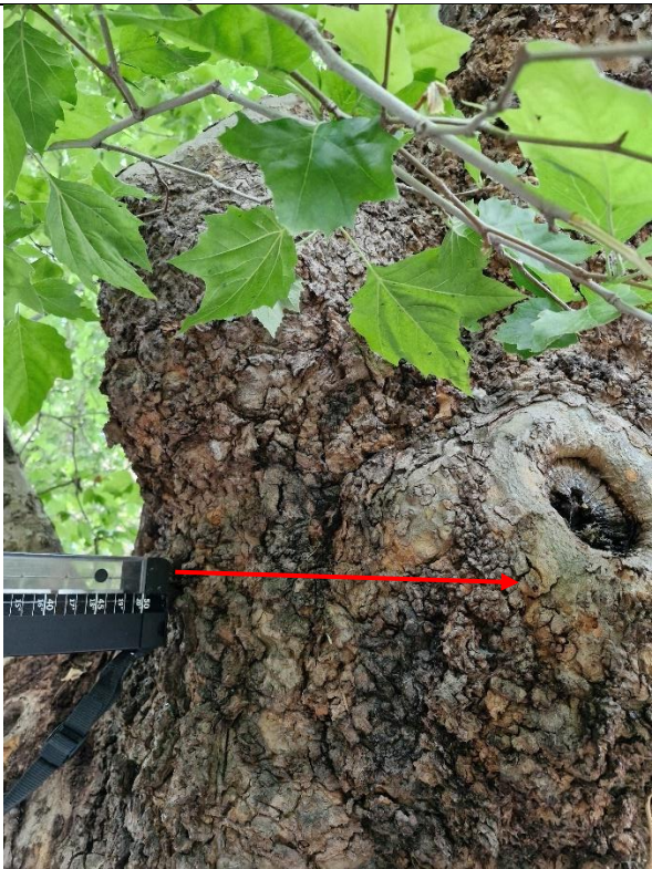
Photo 10: Showing location of resistance drill profile 1 carried out at 4m to the south-west, below the historical wound towards the centre of the stem. Approximate projection of drill shown by a red arrow.
