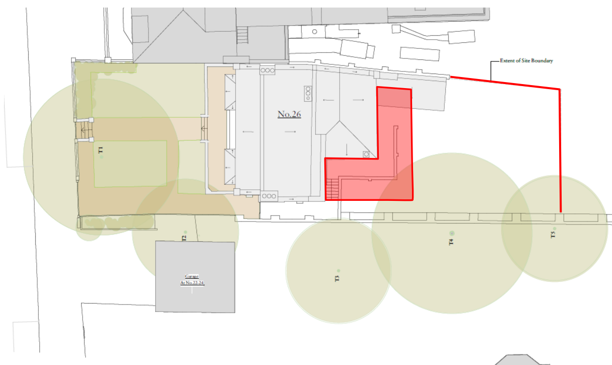
Figure 1: Site baseline plan (21040 EX-00-002) with proposed works areas demarcated within the redline boundary.
