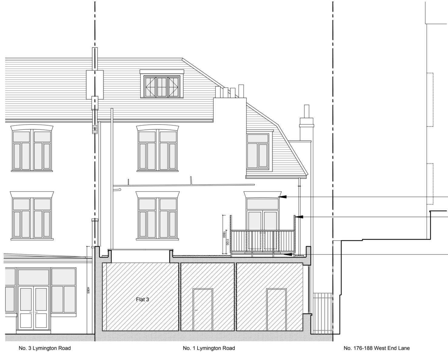
Carefully lower existing window opening to create new door opening to install new double glazed timber french doors
