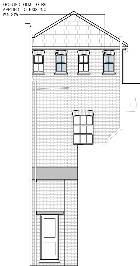
2-6 LEEKE STREET COURTYARD ELEVATION 03
