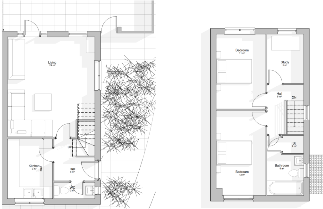
Figure 2: Ground & First Floor Layout
