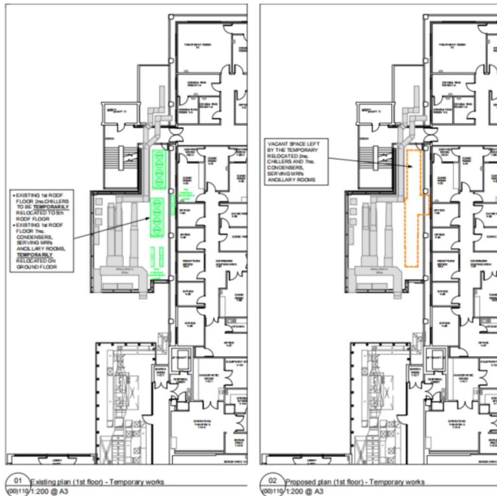
Image 5. Relocation of existing 2no. chillers & 7no. condensing units currently placed on 1 st Roof floor (over MRI-4 suite). The 2no. chillers will be temporarily relocated on the 5 th Roof floor; 7no. condensing units, serving MRI ancillary spaces, will be relocated temporarily on the ground floor.
