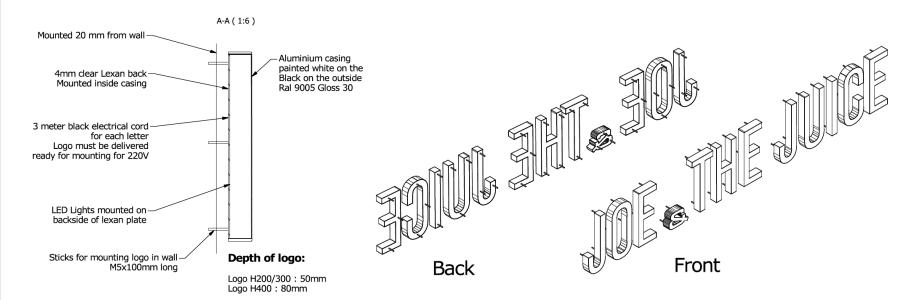
Supplier must place enough sticks on letters to insure mounting of letters in wall. Min 3 sticks per letter. Suplier must deliver logo with a mounting template
