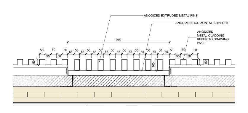
01 ANODIZED METAL FINS GROUND FLOOR PLAN SCALE 1:10 @ A1
