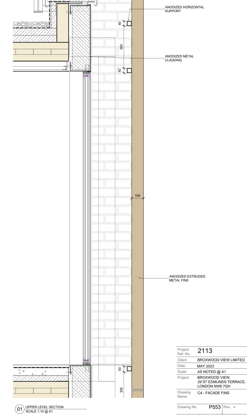
01 ANODIZED METAL FINS GROUND FLOOR SECTION SCALE 1:10 @ A1
