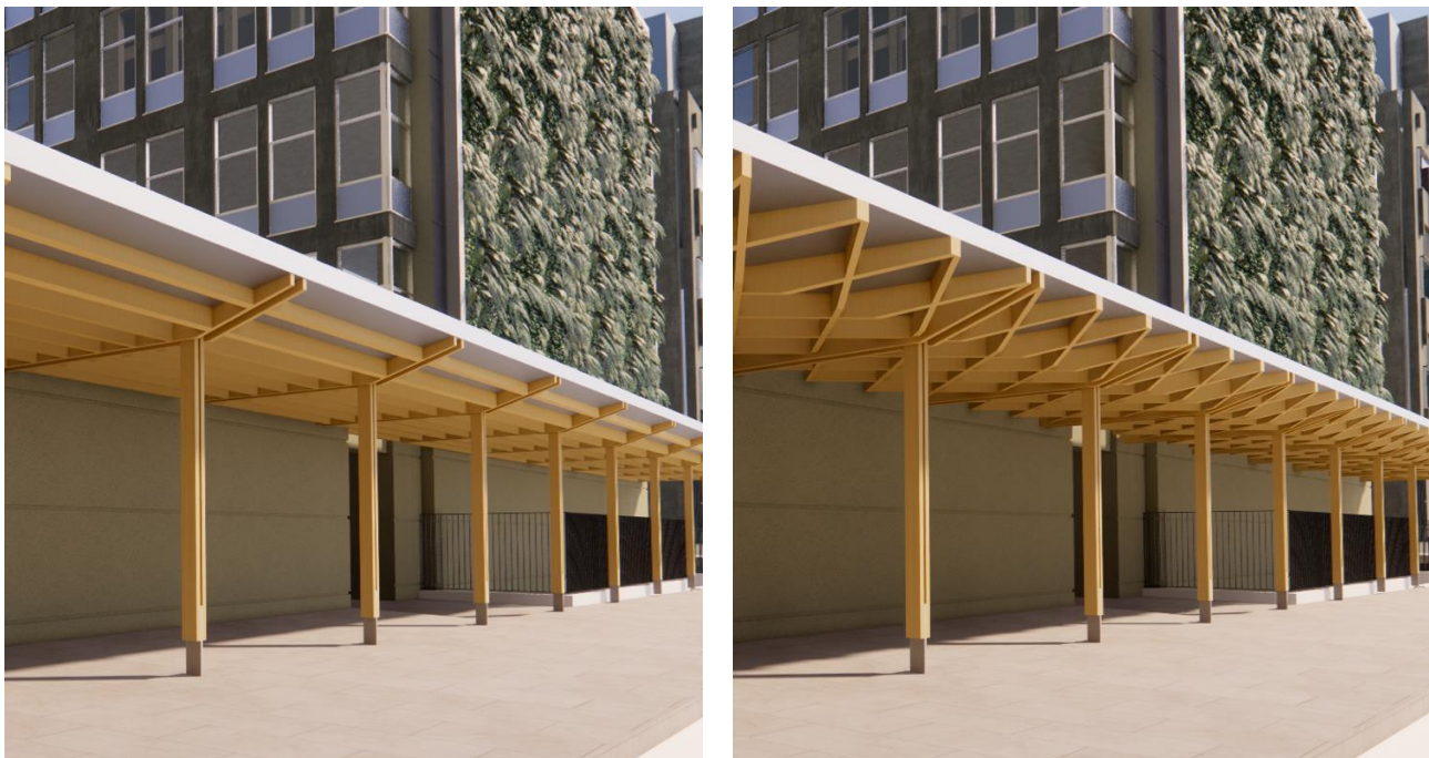
Above: testing different strategies for the canopy's timber structure, which will be designed to have a continuous deck above to protect the timber structure and to support the green and blue roof above.
