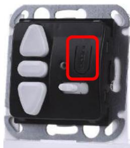
**Step 6:** Press and hold the PROG button back of the remote control, until motor will jog briefly.
