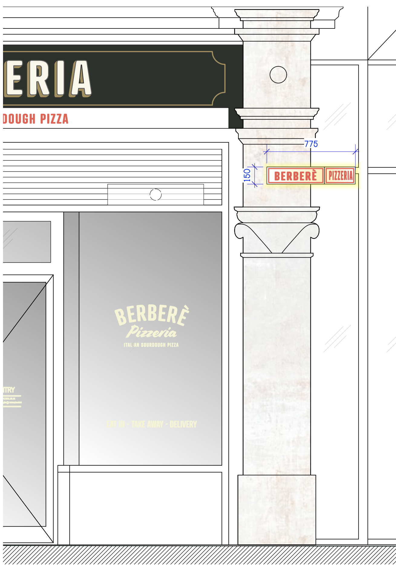
3 Corner Lightbox Detail Front elevation Scale: 1:20
