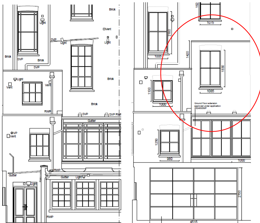
Images 14 & 15: Existing rear elevation (left) and proposed rear elevation (right), with proposed first floor extension sitting on top of existing lower ground floor extensions approved under application 2024/0035/P
