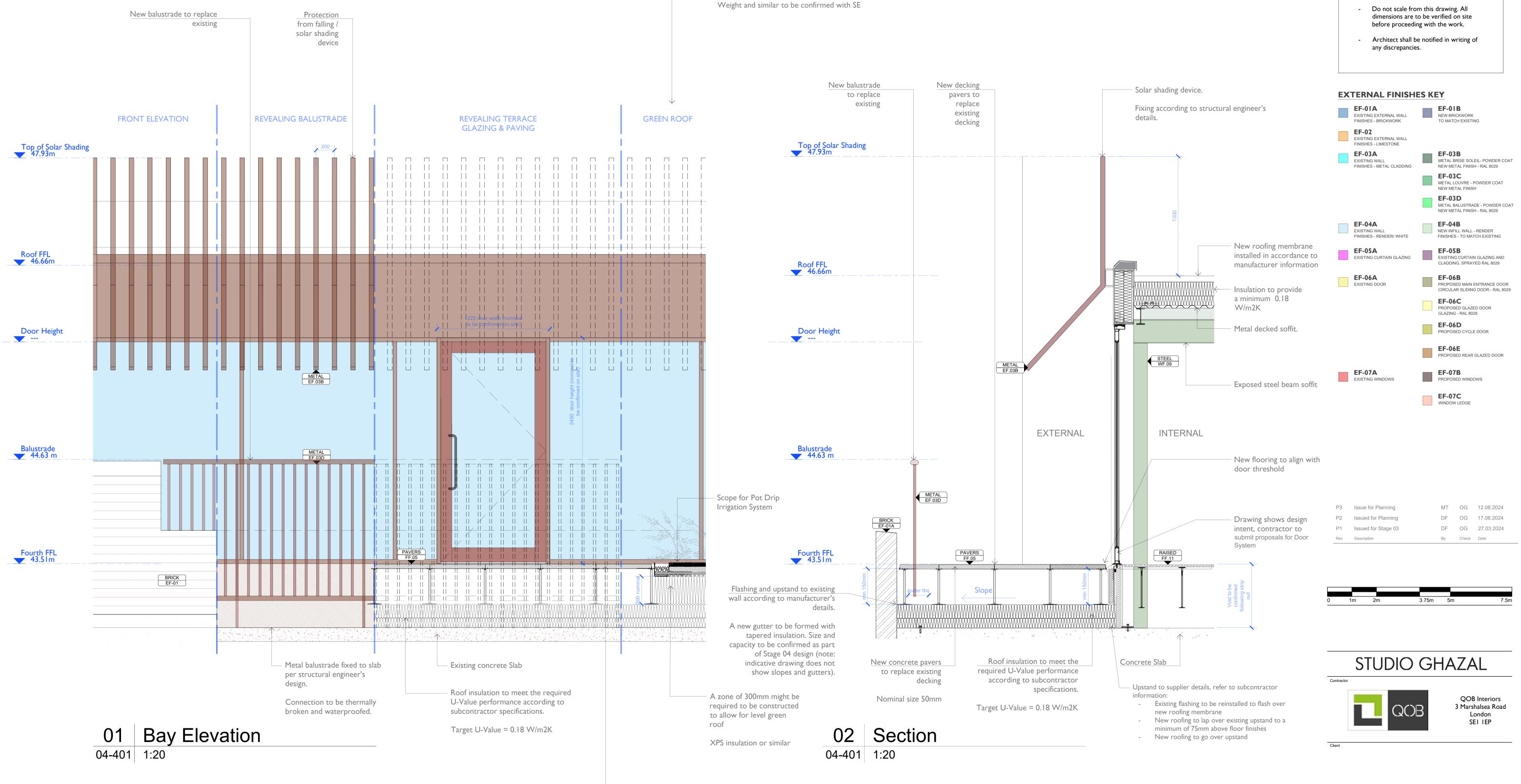
Green roof to be installed nominal build ups Water retention fleece 40mm cuspated water retaining base: Filter layer: 90-120mm growing medium – depending on plant species selection Wildflower blanket Associated retention trims and ballast margins
