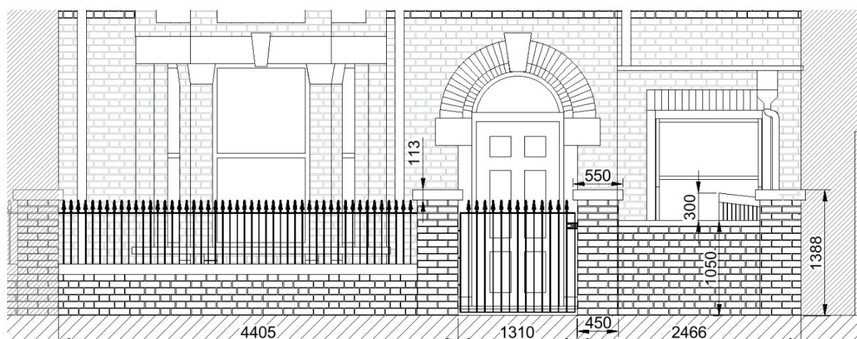
Figure 4 – Proposed wall with dimensions
