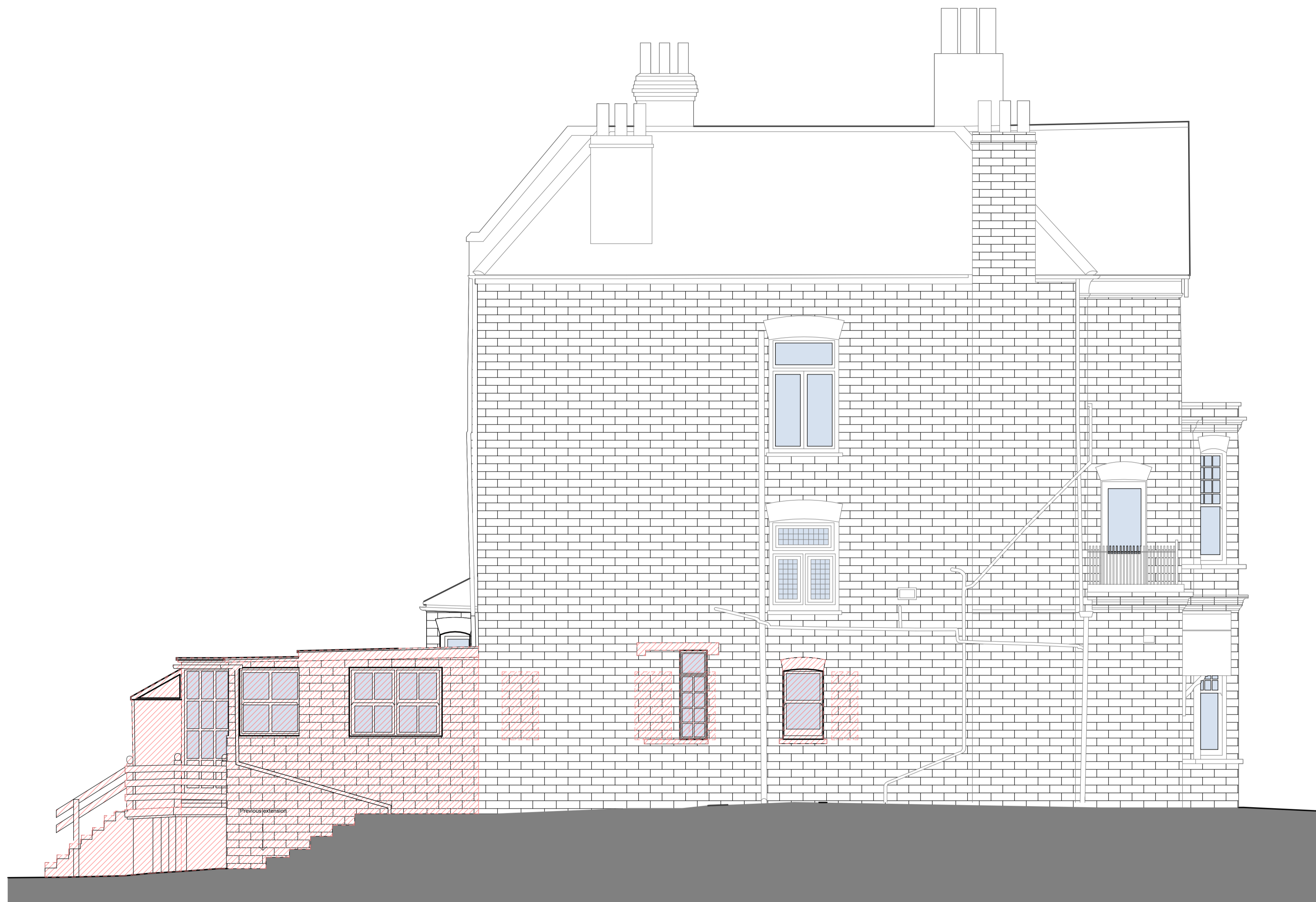
Side Elevation - Demolition 1 : 50
