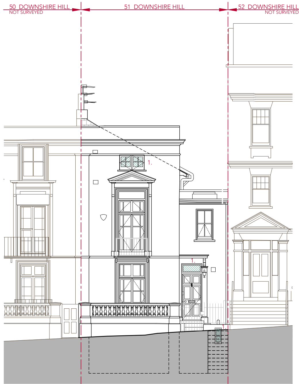
2 FRONT ELEVATION - PROPOSED scale 1:100
