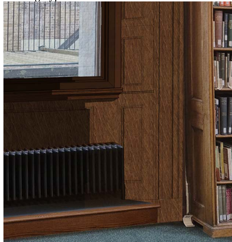
Illustration showing secondary glazing sitting on proposed sub sill
