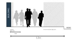
The recommended minimum footway width (total width) for a site with low flows is 2.9 m. This is enough space for comfortable movement and a large piece of street furniture such as guard rail, cycle parking (parallel with the road), a bus flag for a low activity bus stop or a busy pedestrian crossing.
