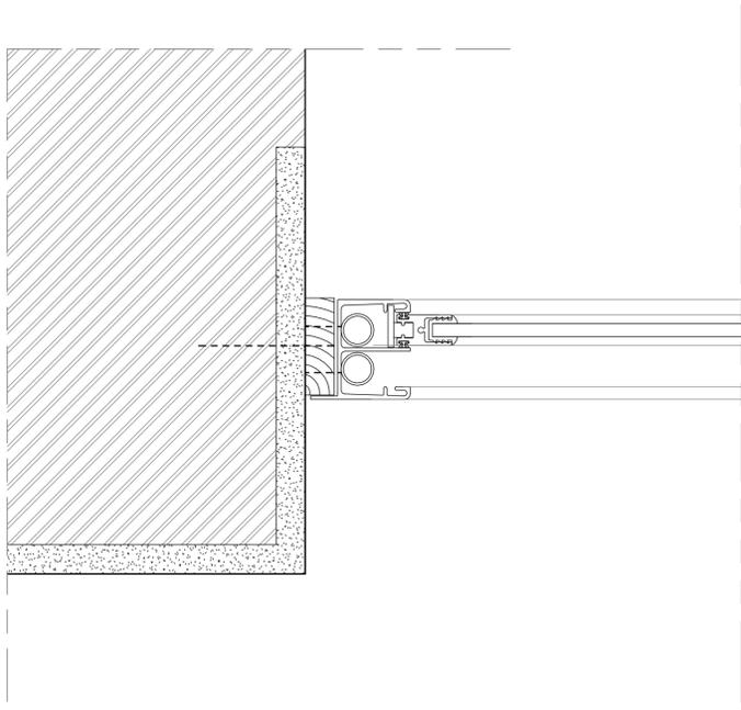
**1 Standard Square Reveal Fixing Detail - Series 25 Unit shown**
