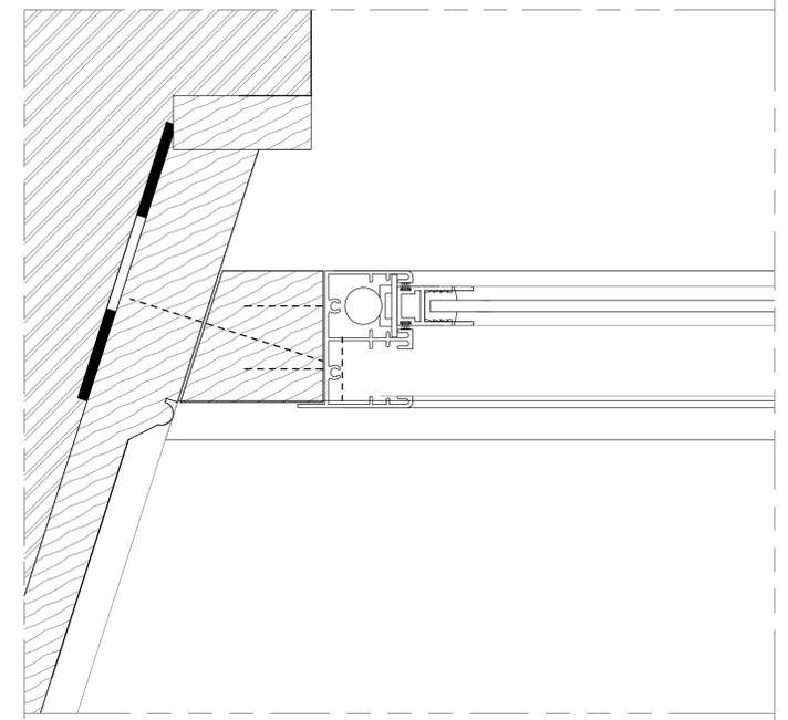
**3 Splayed Fixing Detail - Series 90 Unit shown**
