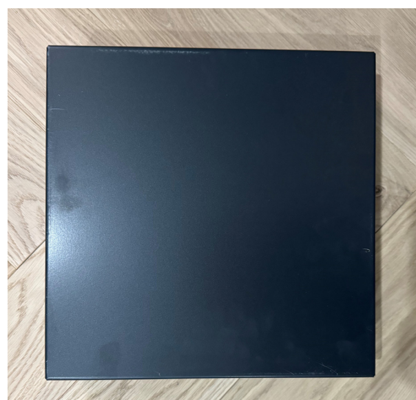
EXTERNAL FACE OF ROOF PLANT SCREEN | RAL 7021
