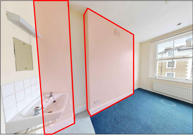
PARTITION DEMOLITION ON BEDROOM 06 & REMOVAL OF EXISTING SINK
