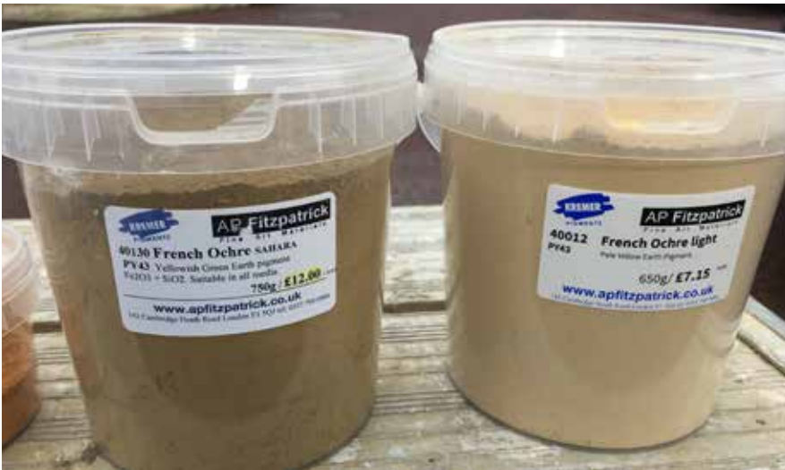
Examples of tinting material used in the repairs.
