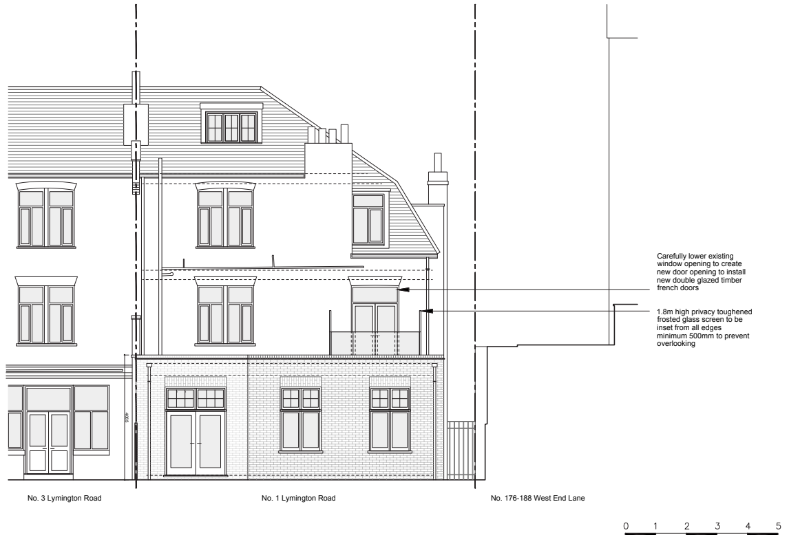
Rear elevation drawing showing the proposed new terrace and French doors.
