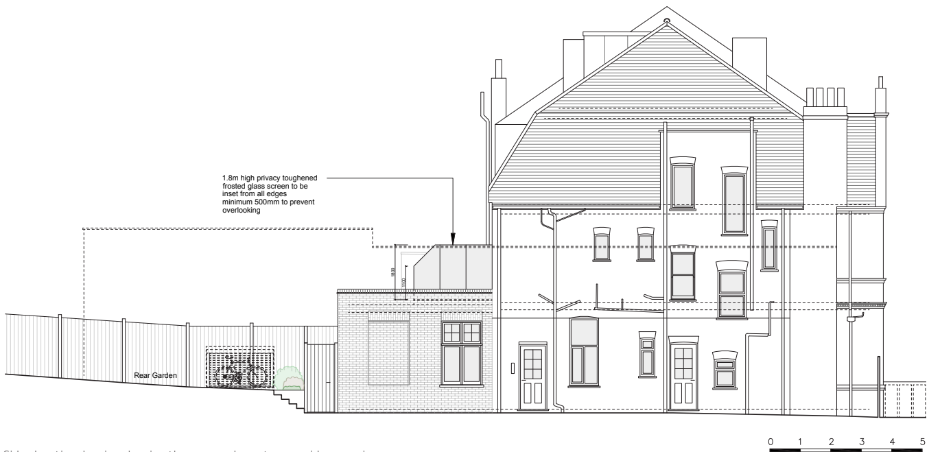
Side elevation drawing showing the proposed new terrace side screening.
