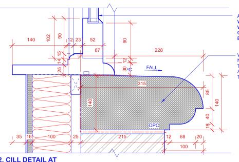
ALL NEW WINDOWS TO MATCH THE EXISTING WINDOWS ARE TO BE FINISHED WHITE AND FITTED WITH DOUBLE GLAZED UNITS TO ACHIEVE A U-VALUE OF1.4W/m²K AS REQUIRED BY THE CURRENT BUILDING REGULATIONS.
