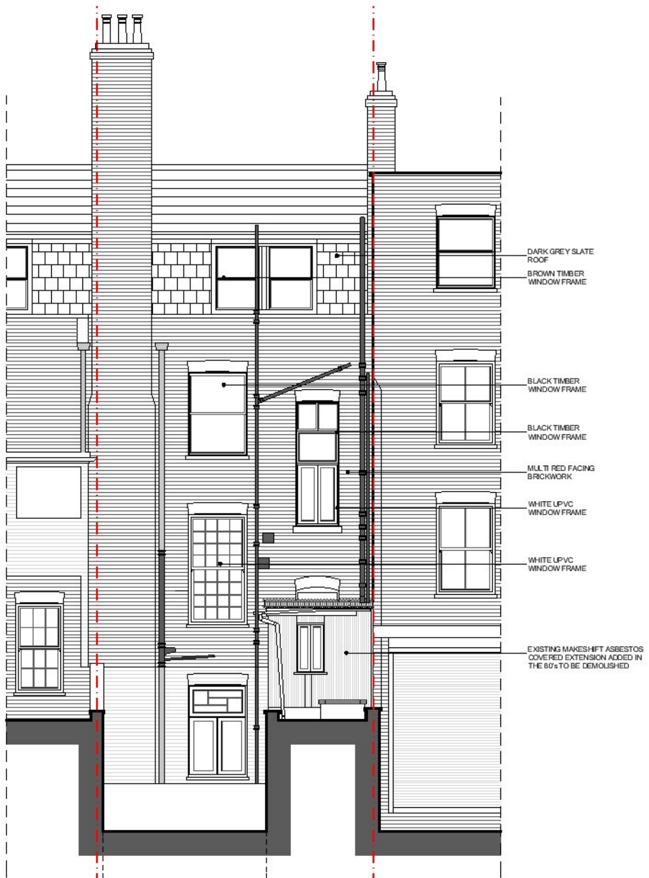
Above: existing rear elevation showing asbestos-covered extension.
