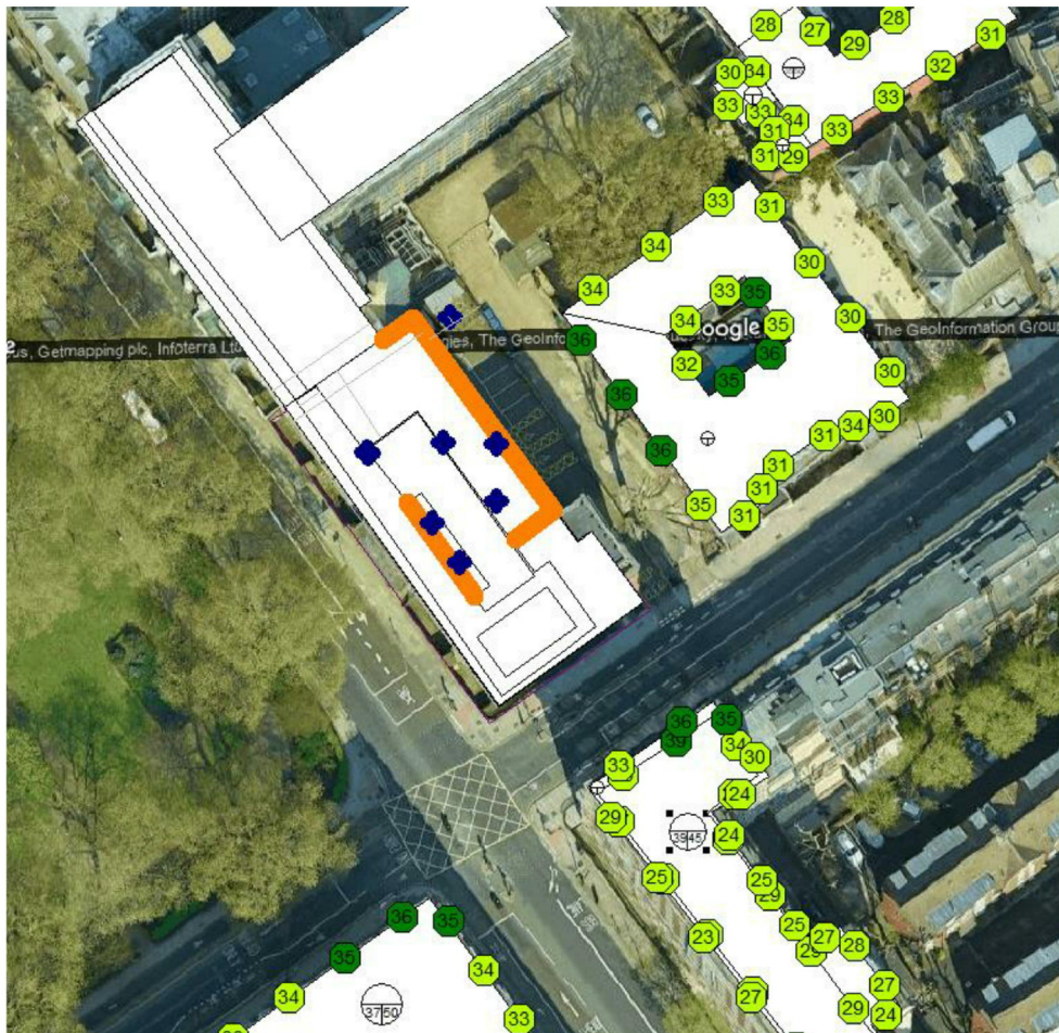
Figure 3: Screenshot of the CadnaA noise model – Acoustic screen (Orange line) and plant location (Blue crosses).
