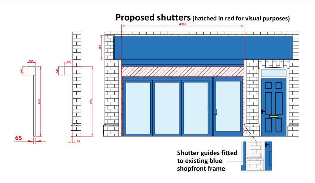
Steel roller shutter, powder coated in white (RAL 9003) with 89mm solid lath, guides fitted to existing shop front as shown above
