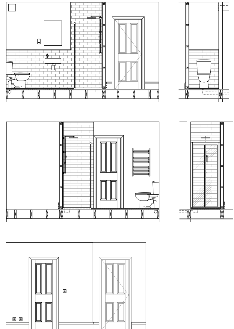
Fig 3 - Extracts taken from planning drawing showing proposed internal elevations of the new en-suite
