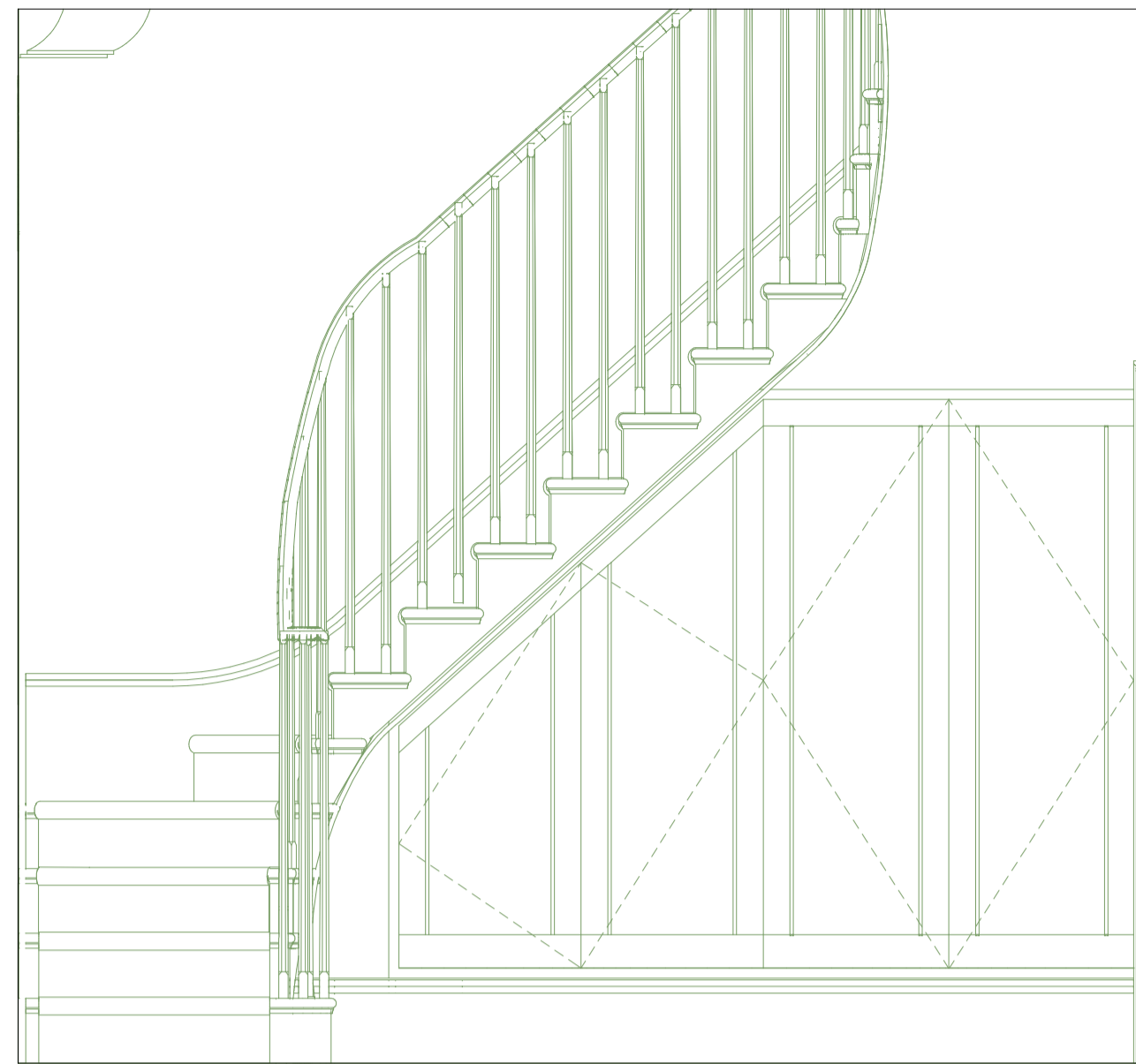
1 L02 Stairwell - Elevation North Wall 1 : 20
