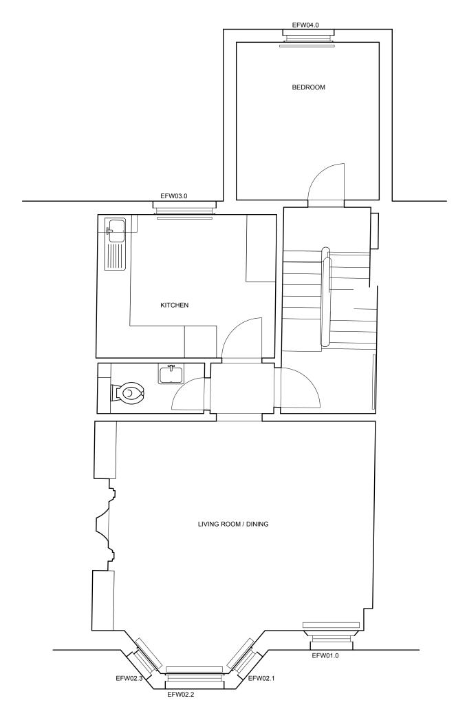
01 FIRST FLOOR PLAN - EXISTING scale 1:50
