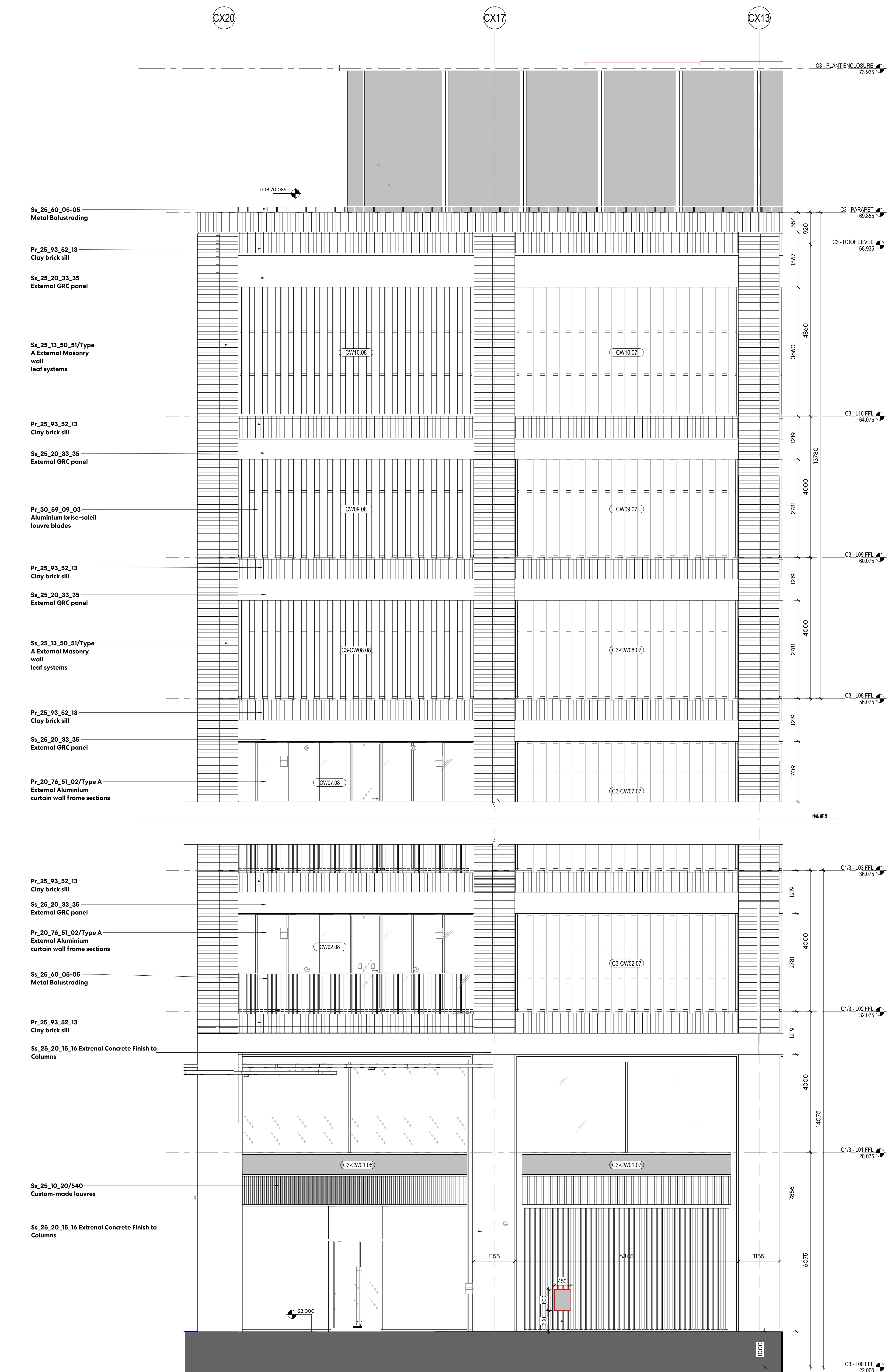
1 C3 - TYPICAL LOUVERED BAY ENLARGED ELEVATION 1 : 50
