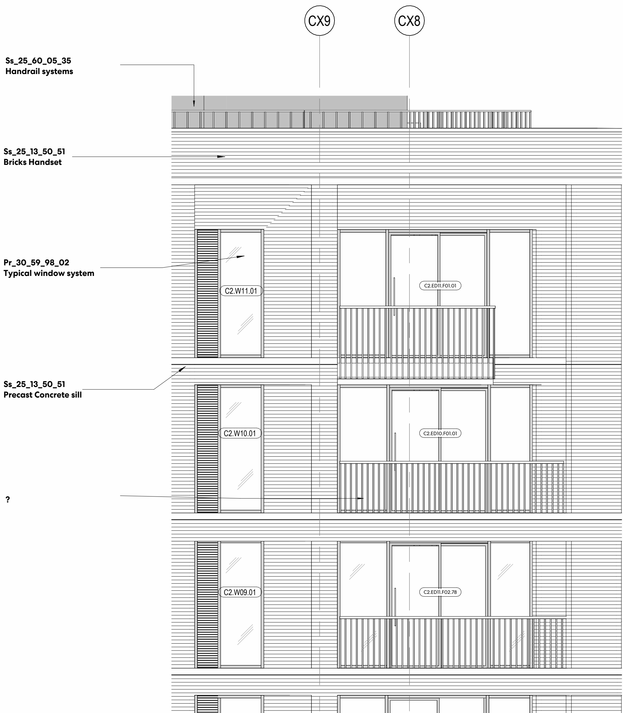
1 TOP CORNER BALCONY ELEVATION 1 : 50
