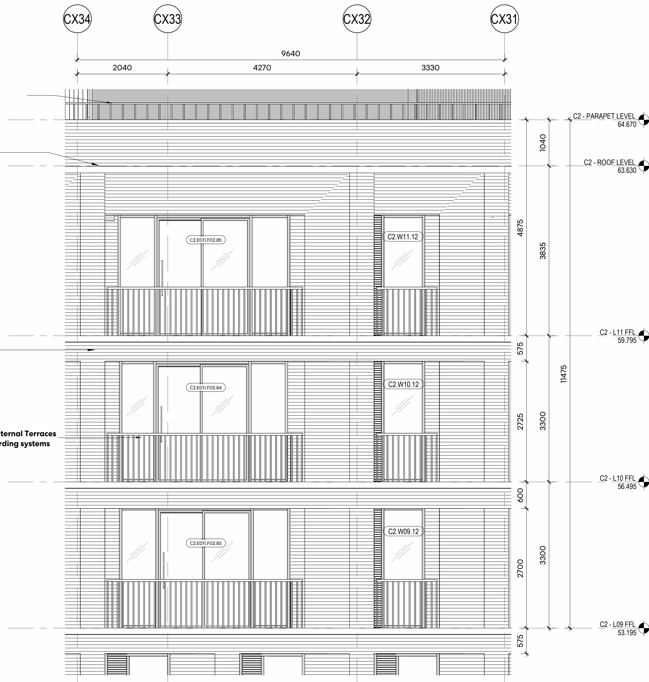
1 BALCONY WEST TOP ELEVATION 1 : 50
