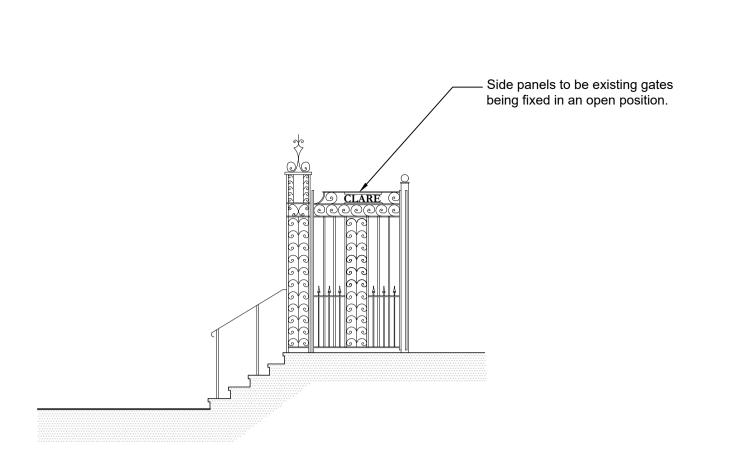
Side Elevation A scale 1:50 @ A1
