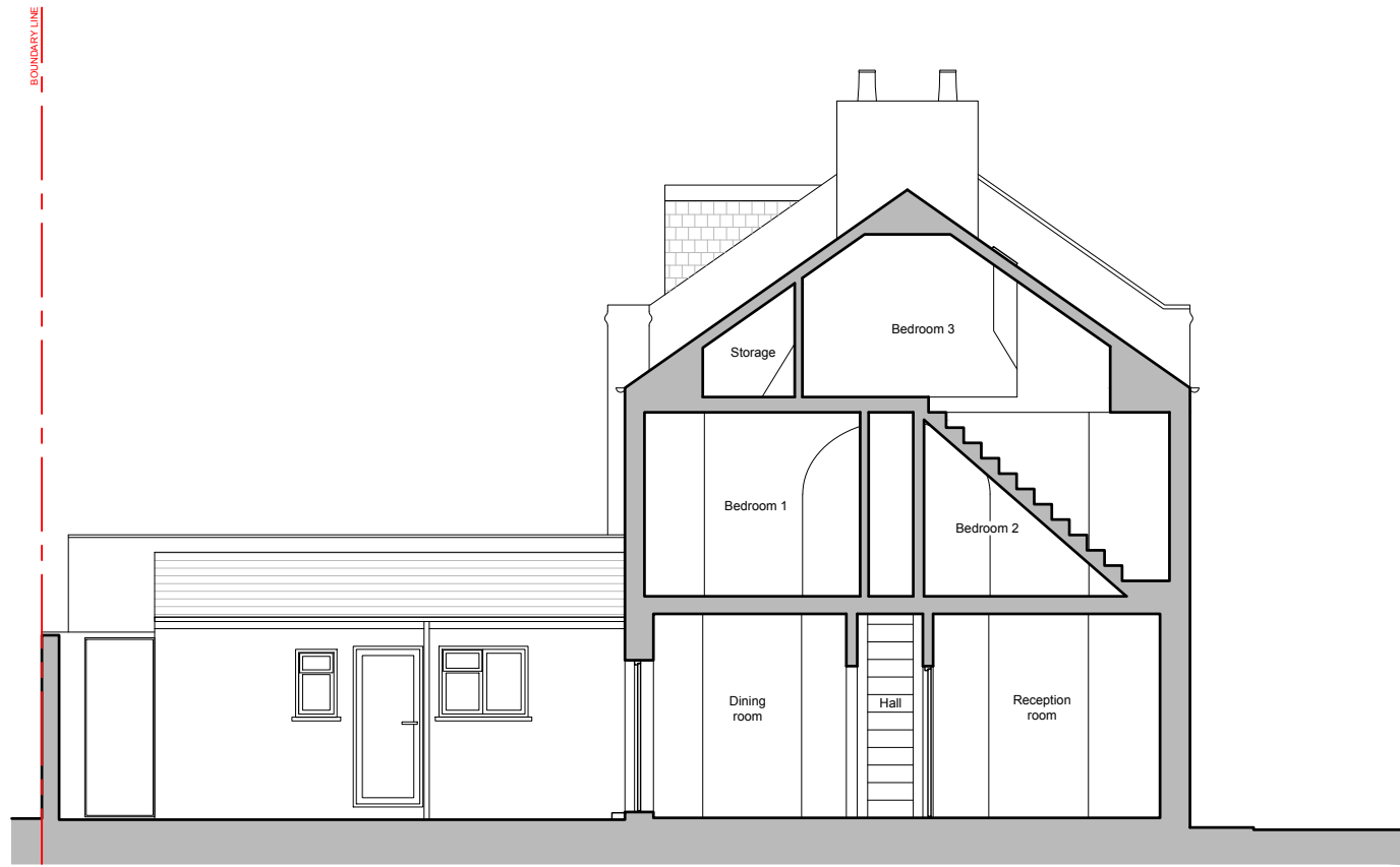
EXISTING SECTION A-A
