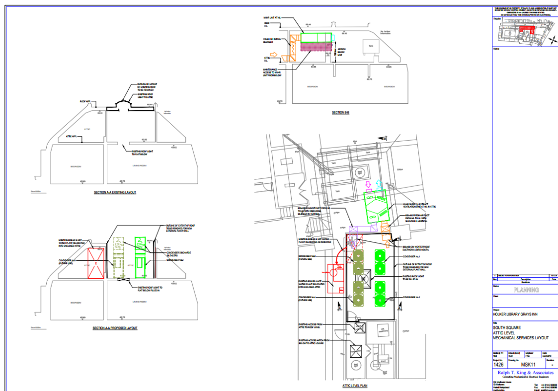
Proposed MVHR and condenser locations within Plantroom 1 indicated on Attic Level Mechanical Services Layout (Drawing Ref. 1426-MSK11)
