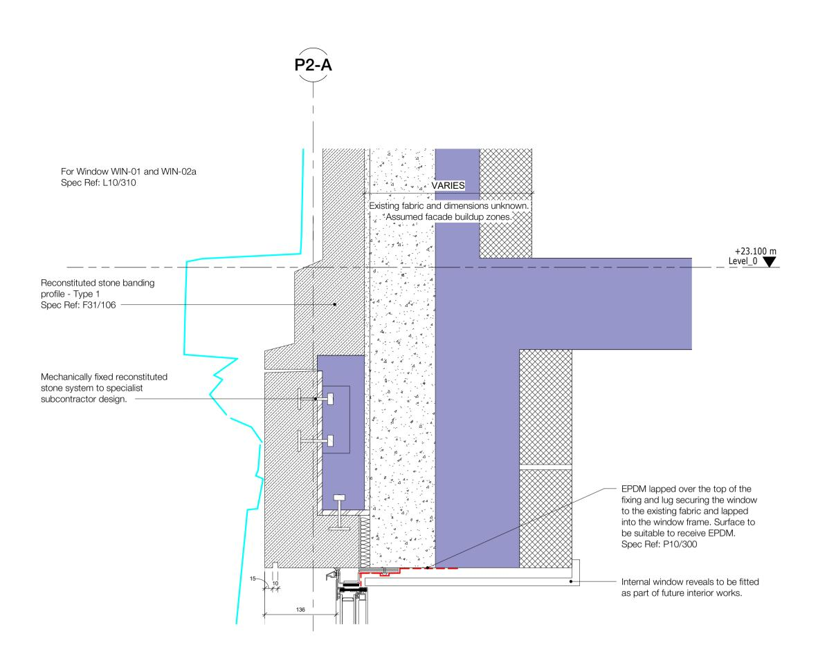
Existing Opening / Typical fixed window head in stone overclad
