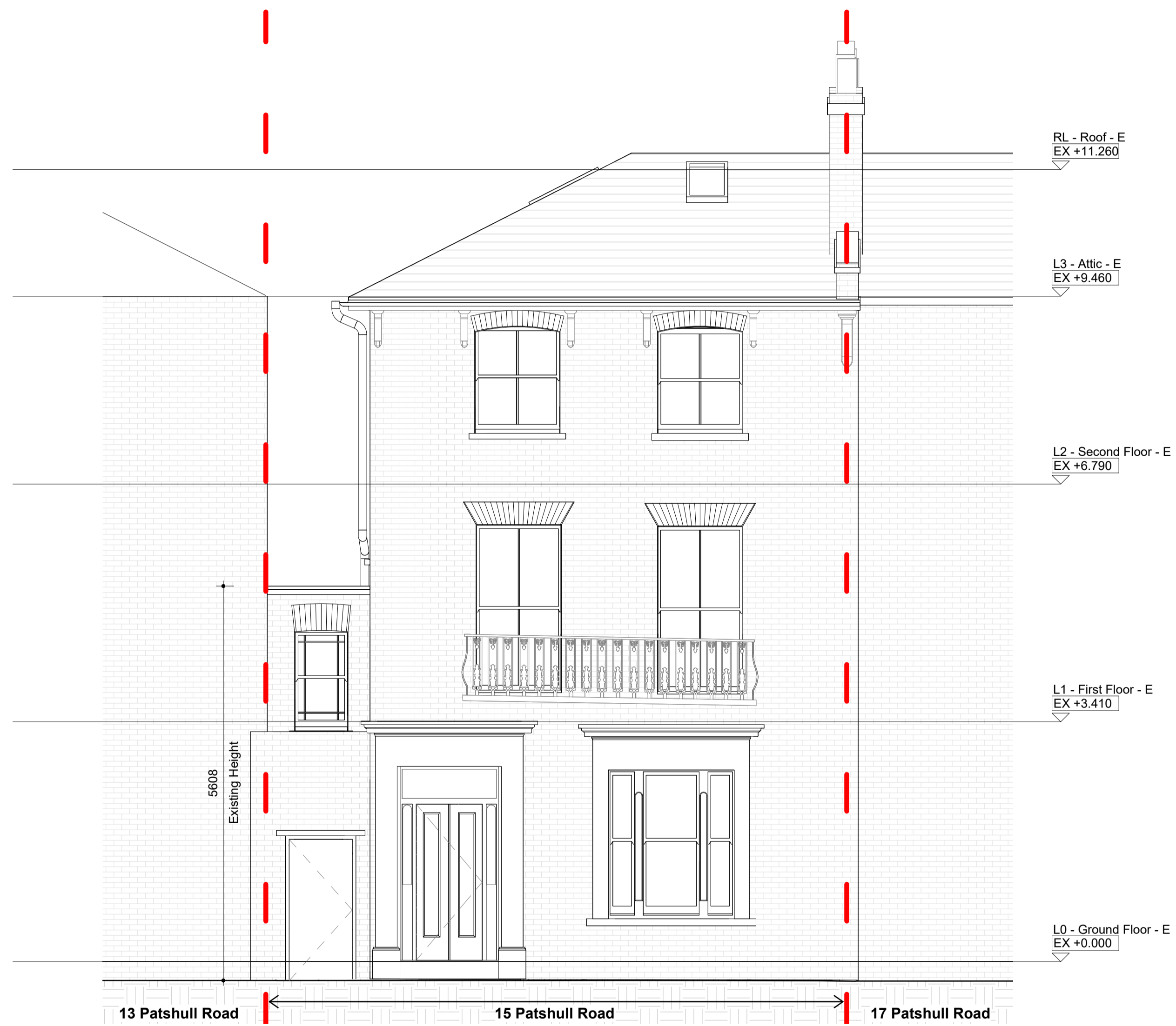
1 Existing Front Elevation 1 : 50
