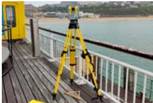
8: Field survey being carried out, total station
