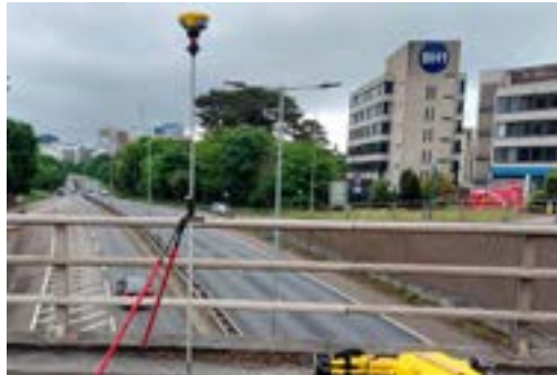
7: Field survey being carried out, GNSS receiver
