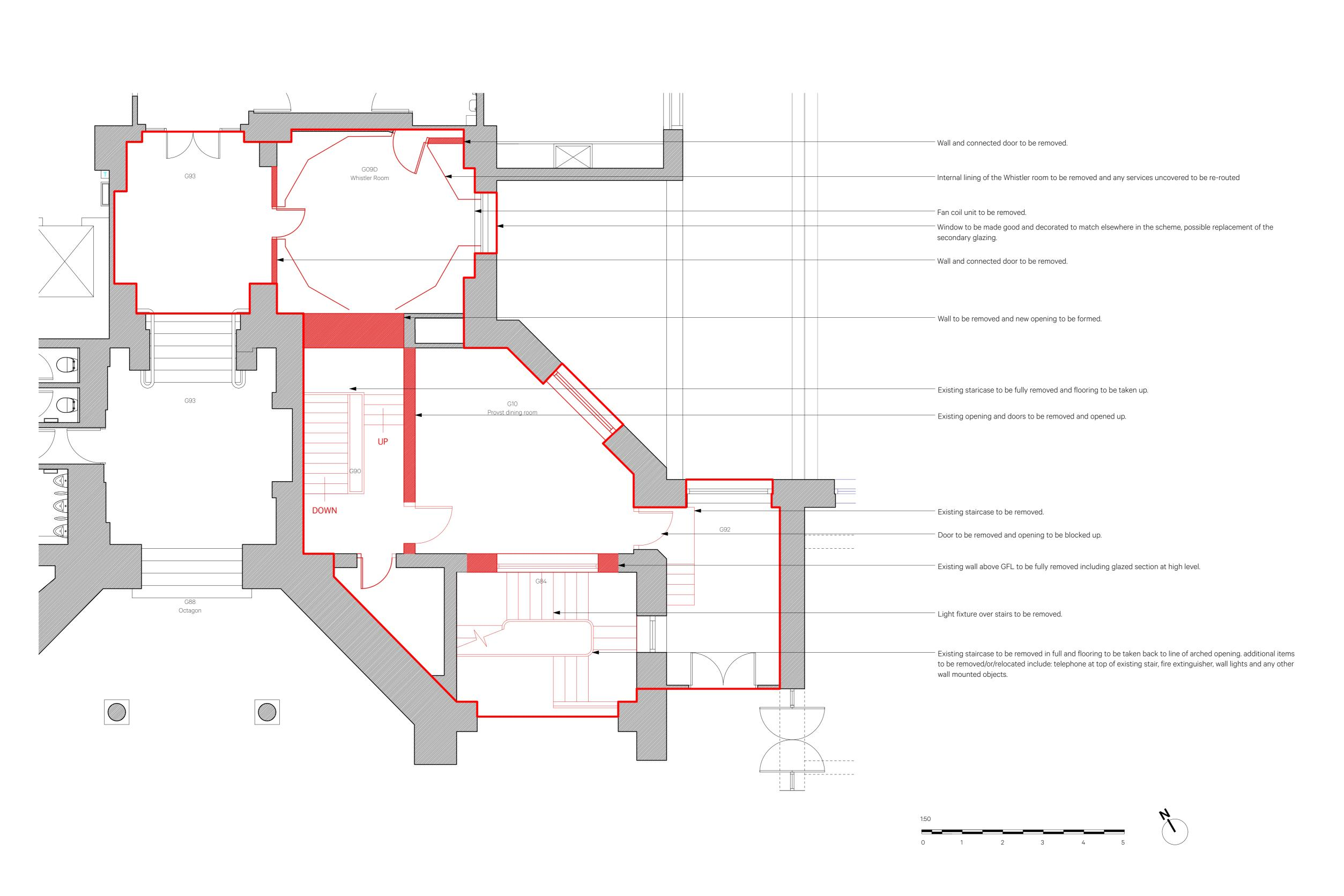
New Lift & Stair - Fabric Removal UGF Plan
