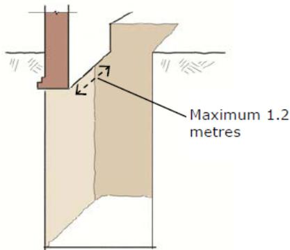
1. Excavation must be fully supported by props and shoring.
