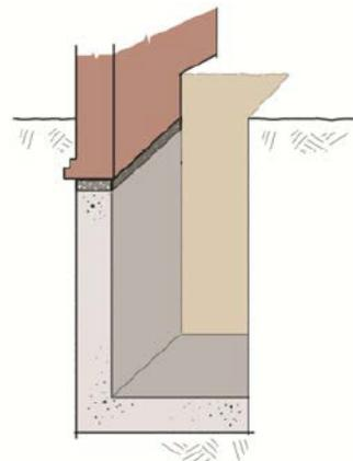
1. After a minimum of 24 hours dry-pack is rammed into the 75mm void that has been left above the new underpin.
