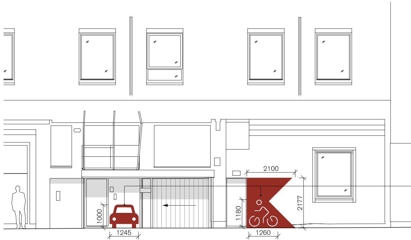
2 Bainbridge St. - Proposed Signage on North Elevation 1:100
