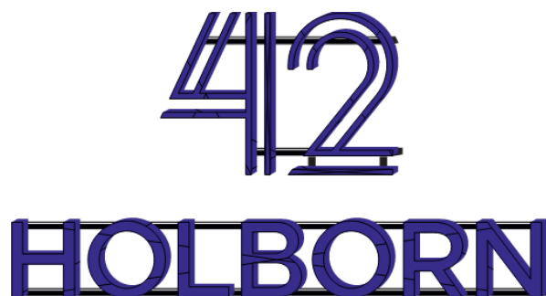
Image 4 – showing proposed non-illuminated fascia sign with horizontal fixing bars
