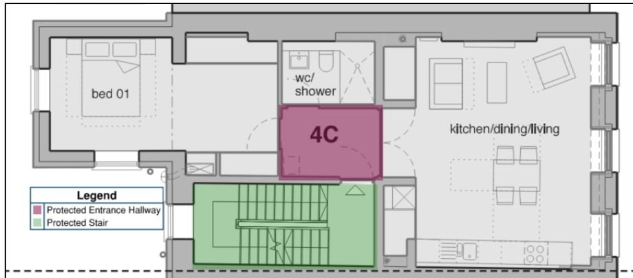
Figure 4: Typical single storey flat layout
