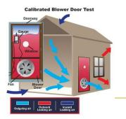
Air tight buildings minimise their heat loss through infiltration of cold air through gaps and cracks in building envelope. Air tightness of buildings is expressed as air permeability rate. Following air permeabilities are targeted in the developments:
