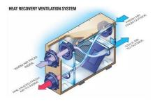
Building regulations Part F recommends mechanical ventilation for dwellings with design air permeability of 5 or less. The most efficient form of mechanical ventilation is the heat recovery ventilation, where warm air extracted from bathrooms and kitchen passes the heat on to the supply air in heat exchanger. Supply air is then distributed to habitable rooms (bedrooms, living rooms).
