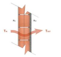
Thermal performance of fabric is the most important aspect of passive measures mosaic. Low U-values ensure, that the amount of heat transmitted through building external elements is minimised. This is achieved by using highly insulated building materials with low thermal conductivity.
