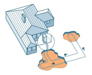
• Vertical loop system can be used where ground space is limited, but will require boreholes typically 15-150m deep, and is consequently more expensive to install than horizontal systems.
