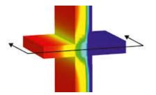
Thermal bridges occur at all junctions between building thermal elements, typically at junctions between wall/floor, wall/roof etc. Recent changes in the building regulations have emphasized the significance of thermal bridging in building design.
