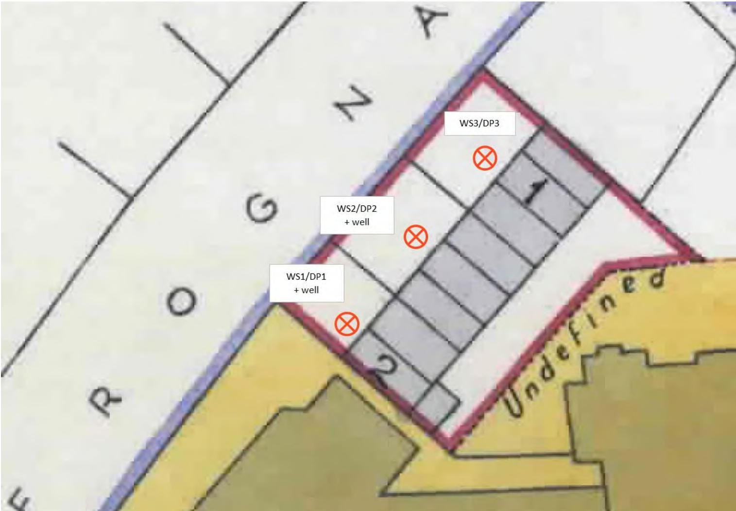
Figure 12 – Exploratory Hole Plan
