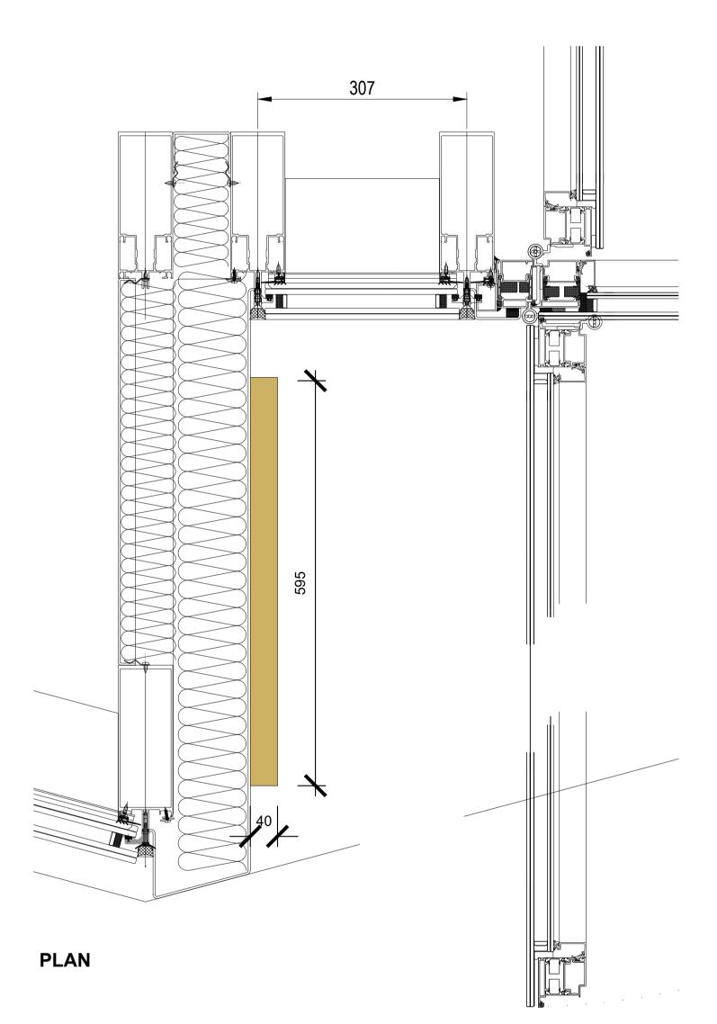
Sign comprising 600mm x 1600mm aluminium sign carcass, finished powder coated Bronze RAL Colour to match existing curtain wall externally.
